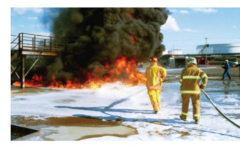
Alcoseal<sup>C6</sup> 3-6 is a superior quality Alcohol Resistant Film-Forming FluoroProtein (AR-FFFP) fire fighting foam concentrate for extinguishing and securing flammable hydrocarbon and polar solvent liquid fires.
