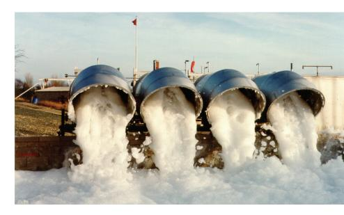
Expandol is a superior quality high expansion fire fighting foam concentrate for extinguishing and securing flammable hydrocarbon liquid fires.
