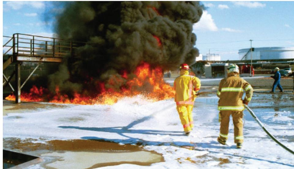
Tridol<sup>C6</sup> ATF 3-3 LT is a cost-effective Alcohol Resistant Aqueous Film-Forming Foam (AR-AFFF) concentrate for extinguishing and securing flammable hydrocarbon and polar solvent liquid fires even at low ambient temperatures.
